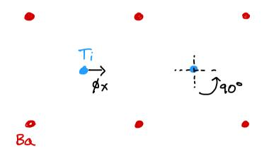
The cubic crystal has various symmetries including  $M_{X/Y}$  and  $C_4 (R_{90^\circ})$ However in (say) Ba TiO3, above some  $T_c$ , the Ti displace by  $\vec{p} = (\vec{p}_X, \vec{p}_Y)$
