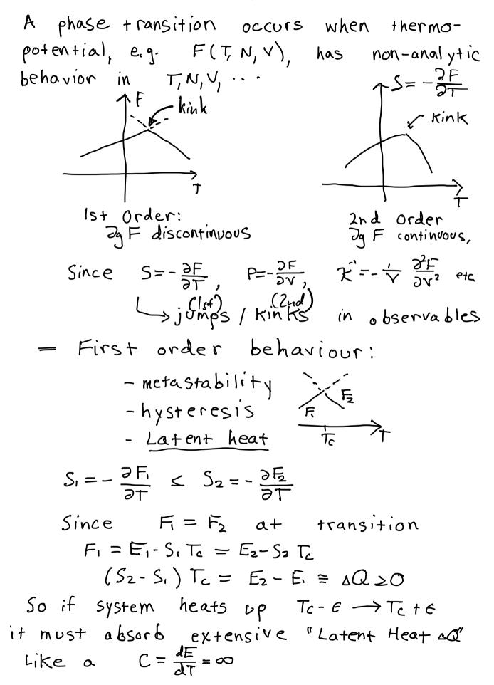
Latent Heat is useful! H20 melting: 334,000 J/Kg = 0Q 6 TECATE Beer phase // Ice phase -Water phase
