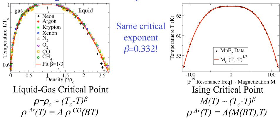
Universality: Same Behavior up to Change in Coordinates  $A(M,T) = a_1 M + a_2 + a_3 T + (other singular terms)$ Nonanalytic behavior at critical point (not parabolic top) All power-law singularities ( $\chi$ ,  $c_{\nu}$ ,  $\xi$ ) are shared by magnets, liquid/gas (Non-symmetric Models: \$3)
